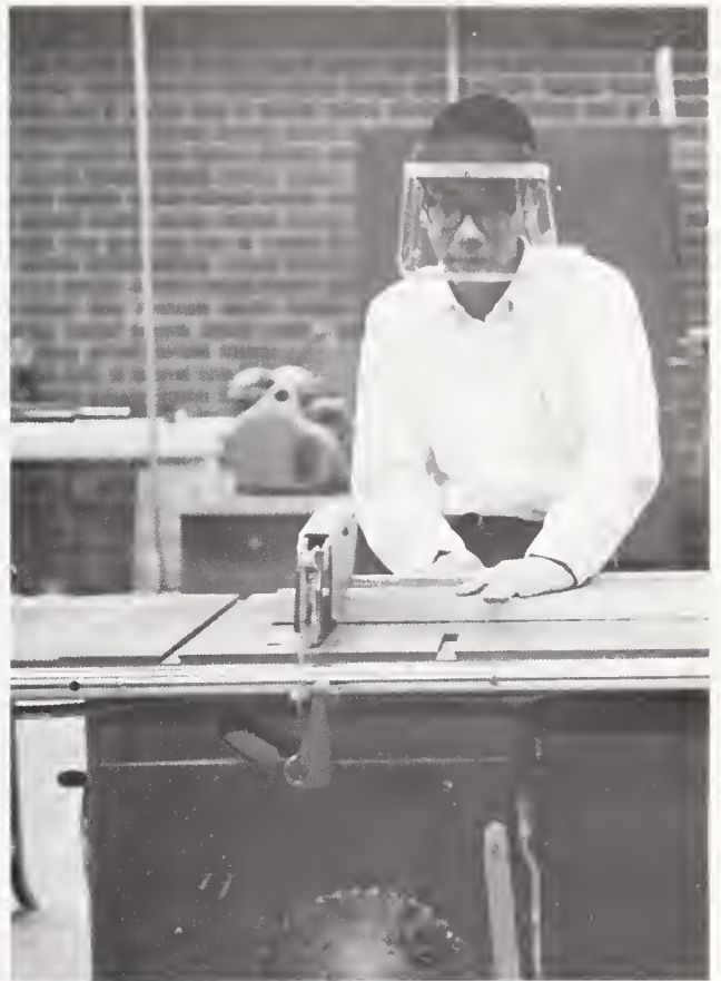
Richard Wong demonstrates the use of a table saw. The mask which is worn is a protective measure to prevent foreign objects from hitting the face and eyes.
