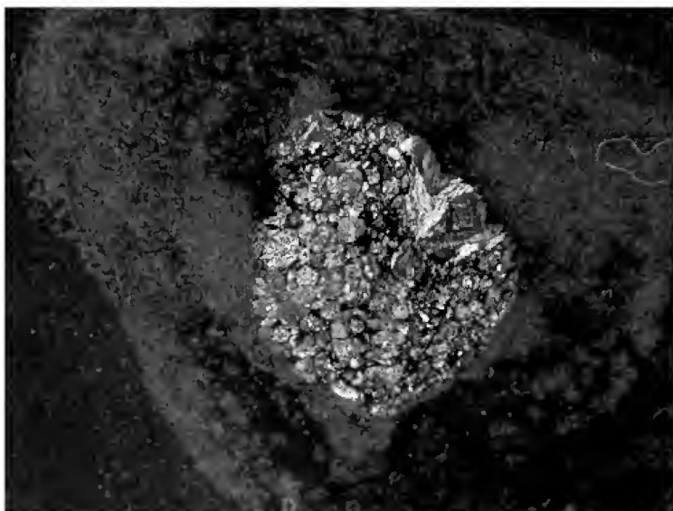
Fig.15- Transmitted crossed polarized light photomicrographs showing zoning olivine crystal. The zoned color range from the crystal's rims to the center of the crystal is an indication of zoning characterized by the change in the mineral composition. Length of field 0.45mm.
