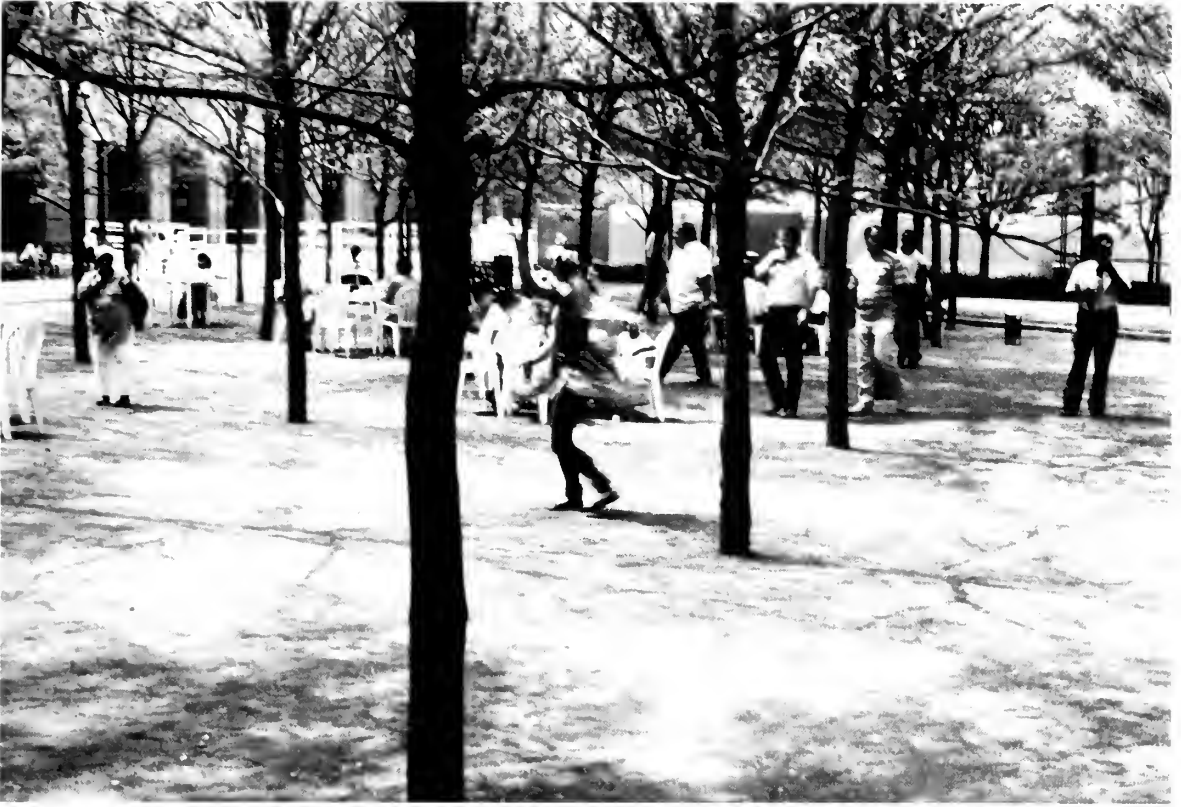
Trees in downtown Brooklyn, NY, planted in paving using a soil mixture with expanded slate aggregate to prevent loss of pore space under compaction from heavy pedestrian use.
