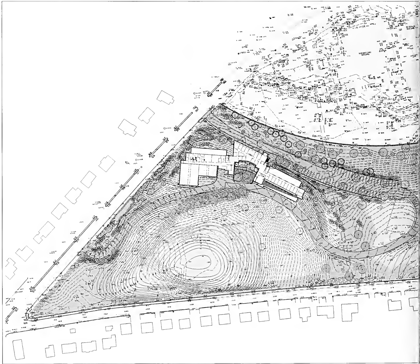
Figure 2. Site plan with topographic detail and building footprint for the Weld Hill facility, by Reed|Hilderbrand.
