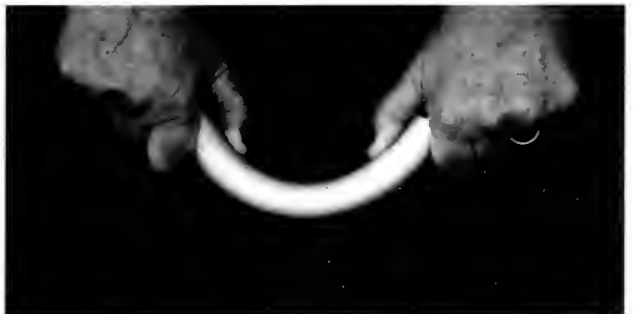
An empty tube kinks when bent, but the foam-filled tube resists kinking.
