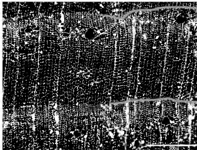
(Left) Sugar maple ( Acer saccharum ) wood, in transverse section (scale bar 500 \mu\text{m} = 0.5 mm); growth ring boundary is marked with red line. (Right) Black pine ( Pinus nigra ) wood, in transverse section (scale bar 500 \mu\text{m} = 0.5 mm); growth ring boundaries are marked with red lines.
