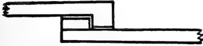
FIG. 153—LOCKING ENDS OF PORTABLE FENCE PANELS This drawing shows manner in which ends of portable fence panels are locked. Also see Fig. 155.
