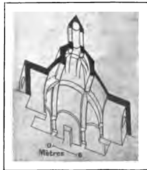
FIG. 75.—RIBBED CUPOLA OF THE CHURCH OF AKHPAT.
