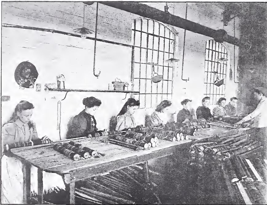
THE THREADING ROOM. SECOND PROCESS IN MANUFACTURE OF AXMINSTER CARPET. No. 4.
