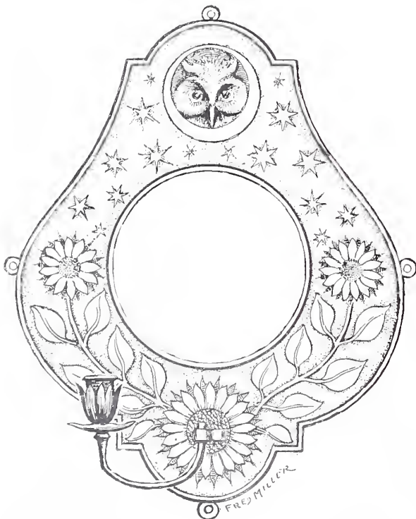
No. 4.—Original Design for Candle-holder with mirror or plain metal in centre. The stars and leaves in low relief, while the flowers and owl in higher relief.
