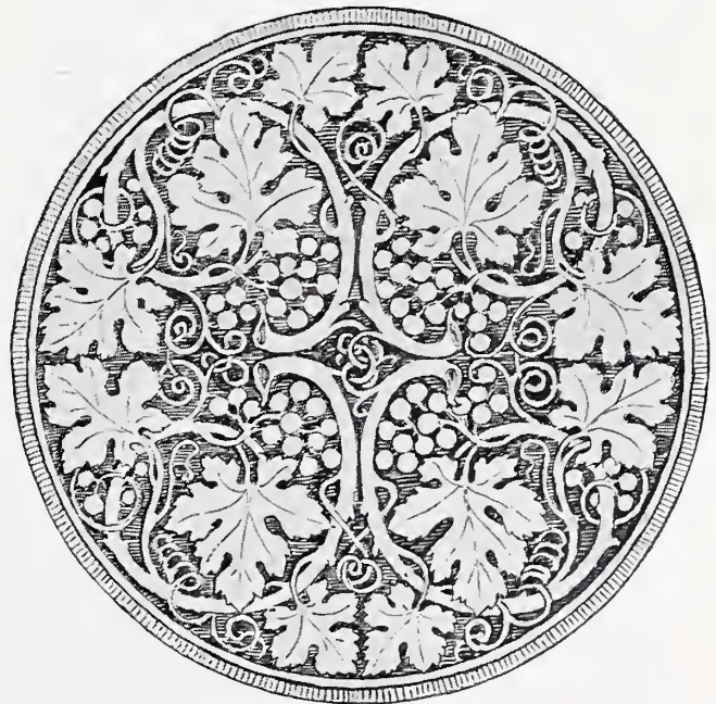
No. 2.—Sketch Design for carved table-top in which the Vine is used as the motif. The work is kept entirely flat, the effect being obtained chiefly by the "grounding-out," for beyond the veining of the leaves and the slight cutting away of one form to give relief to another coming against it, the actual carving ends there. It would be possible to treat this design as a carving in low relief. By planning the design geometrically it matters not from which side it is seen.
