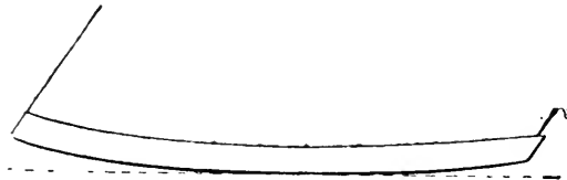
FIG. 48.—Shoe fitted to a curved foot-surface.
