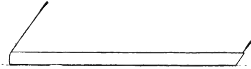
FIG. 49.—Level shoe fitted to level foot-surface.
