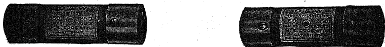
Figs. 1,188 and 1,189.—D and W. enclosed or cartridge fuse showing blow indication. When the fuse blows, it is indicated by the appearance of a black spot within the circle on the label as in fig. 1,189. Fuses should be placed wherever the size of wire changes or wherever there is a branch of smaller size wire connected, unless the next fuse on the main or larger wire is small enough to protect the branch or small wire, but more lights may be added on the large wire, making it necessary to put in a larger one. Experiments have shown that for large fuses, a multiple fuse is more sensitive than a single one. A one hundred ampere fuse may be made by taking four wires of twenty-five amperes capacity.
