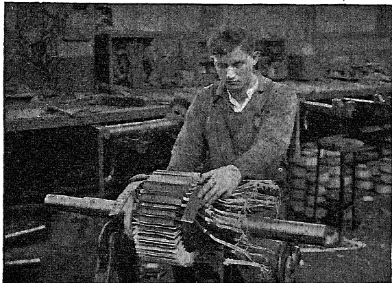
FIG. 1,013. — Reliance motor construction 21. Slot cell insulation which extends \frac{1}{2} in. beyond the core. Note strips of press board taped into continuous rings which insulate top and bottom layers of armature coils at the head.
