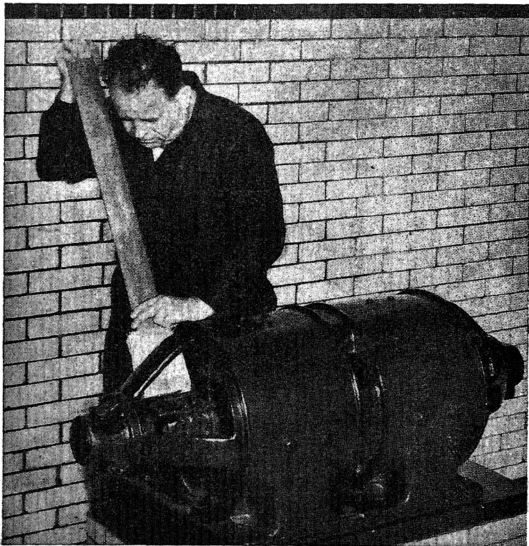
FIG. 929-13.—Method of application of canvas wiper to commutator. Holding the strip at right angles to the machine shaft is usually the most convenient method of application on small machines. (Courtesy National Carbon Company, Inc.)
