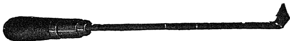
FIG. 929.—Commutator hand scraper. This tool is for removing mica fins which are left in the slot by the grooving saw. A triangular curved file is sometimes used for removing the copper projections, but the removal of a very thin portion of the commutator surface by turning in a lathe, using a special high speed steel tool (trade name No. 3 Stellite) is recommended. The remaining copper burr left on the trailing edge of each commutator bar can be removed by the hand scraper above illustrated. A final polishing with sandpaper will make a smooth surface which is necessary for good commutation and long life of brush.
