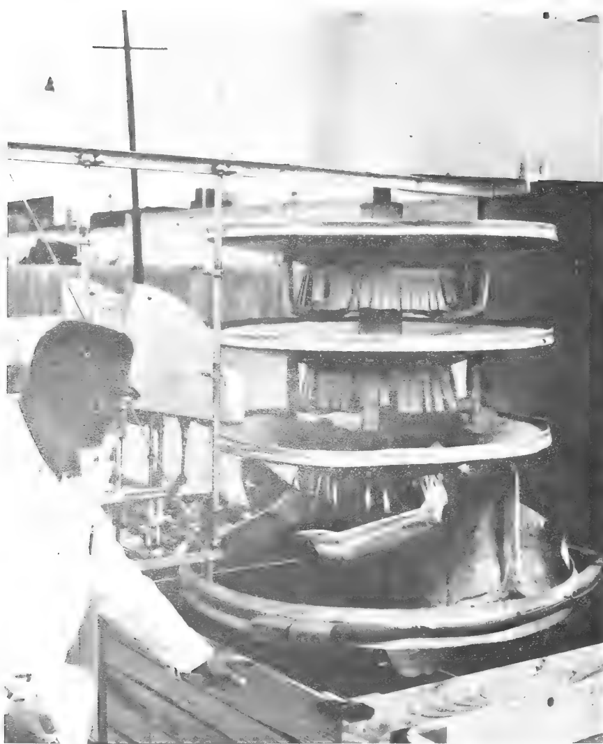
Figure 19.—Filler in raised position ready to be lowered into pallet box.
