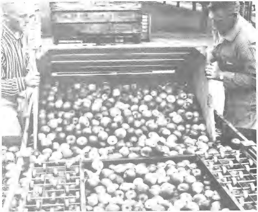
Figure 25.—Start of water dumping of pallet box.
