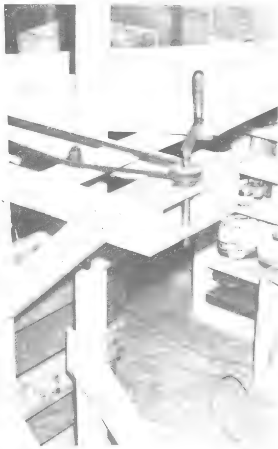
Figure 4.—Wooden frame used for filling distribution study.
