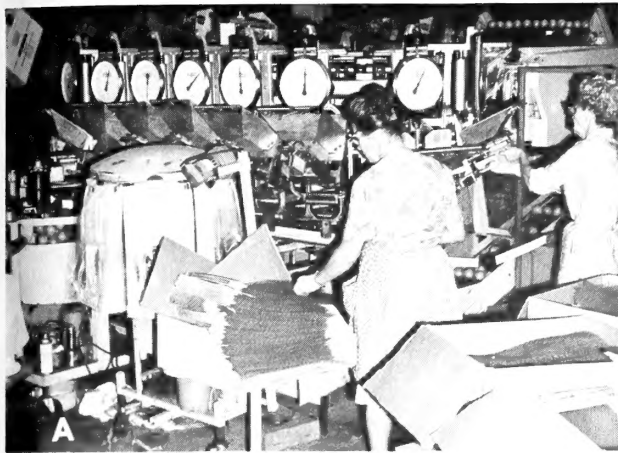
Figure 4.—Carrousel bagging machine. (Top) Workers hanging polyethylene net bags on filling heads. Device for automatic hanging of polyethylene film bags at left foreground, loaded with bags on wickets. (Bottom) Filled bag discharge. Worker at left is check-weighing and worker at right is attending the automatic staple-closing unit.
