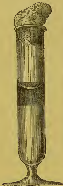
FIG. 2. Eprouvette used in this and the following experiments. It is plugged with cotton wool and charged with test liquid, to which distilled water has been added in the prescribed proportion, so as to avoid mixing. After standing a week the upper layer, with which distilled water is mixed, has become turbid.
