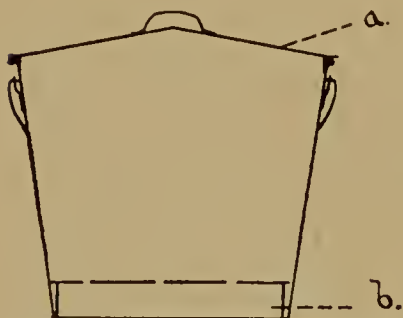
FIG. 3. Simple sterilizer consisting of a galvanized iron pail with a cover a and a false bottom b .
