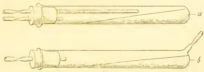
FIG. 26.—Tubes for anaerobic cultures on the surface of solid media.
