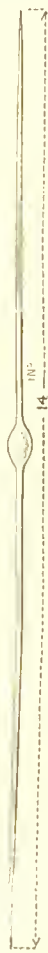
FIG. 5.—A CAPILLARY PIPETTE, DRAWN OUT INTO FINE POINTS: LENGTH ABOUT 12 TO 14 INCHES.
