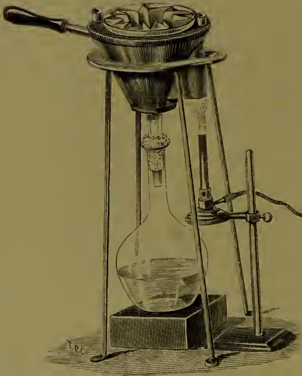
FIG. 6.—HOT-WATER FILTER FOR FILTERING NUTRITIVE GELATINE OR AGAR-AGAR MIXTURE.
