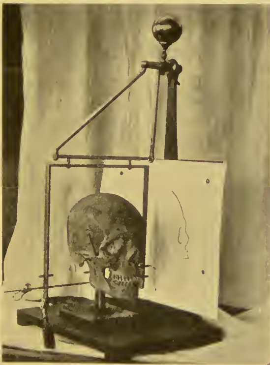
Fig. 7. The stereograph of Broca: a mechanical device for producing rectilinear projection drawings of crania or similar objects. For further description see Chapter x.
