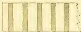
Wood, with the Strips glued on.
