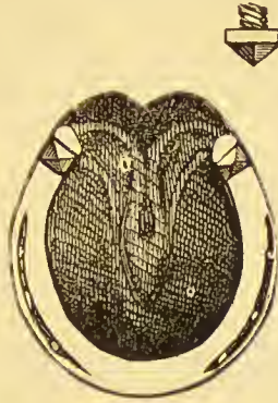
A SHOE, WITH POINTS, WHICH SCREW ON AND OFF, DESIGNED TO FIT A HORSE FOR WORK DURING FROSTY WEATHER.
