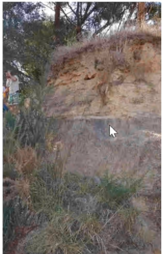
Graphic examples from Tarawingee (left) and Garibaldi (right). The sludge layer is the lighter coloured upper layer more than a meter above the darker native soil of the 1880 level.
