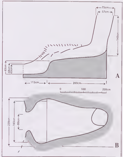
Fig. 6. A, lateral; and B, plan view of the Intaken kiln showing the free-form shape with the chimney at a slight lean and off-set to the side, indicating that it was excavated rather than constructed. The dotted line indicates a small fire hardened arc that was a section of the circular firing pit, rather than a jar-like rim to the kiln itself as interpreted by Prishanit and Suphamas (1997).
