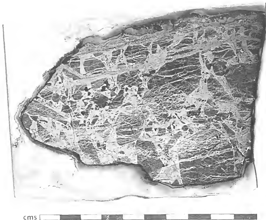
Fig. 2. Polished section of an apparently massive hand-specimen of iron shale (NTM 821-26). The pallasite structure is preserved though iron oxides have invaded fractures in the olivine crystals. The dominant crystal-fracture direction (left to right in the photograph) produces a planar fabric. Such specimens are not fissile along these planes.
