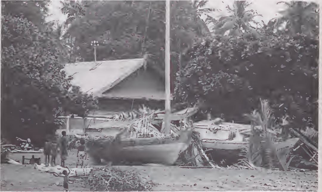
Fig. 13. Large juko with a shallow, beamy midsection.
