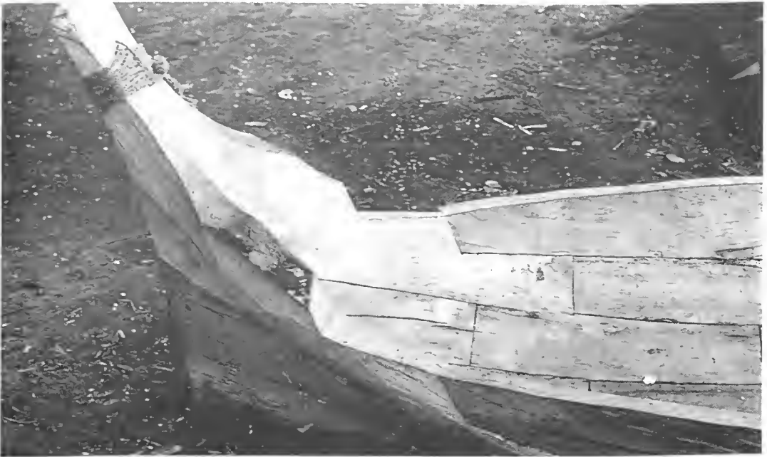
Fig. 5. The bow of a sapa under construction showing the roughly shaped to'bo .
