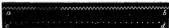
FIG. 30.—GRAPHIC REPRESENTATION OF RATE OF VIBRATION OF BEE'S WING. a , b , Line Made by Tuning Fork; c , d , Marks Made by Vibrating Wing.
