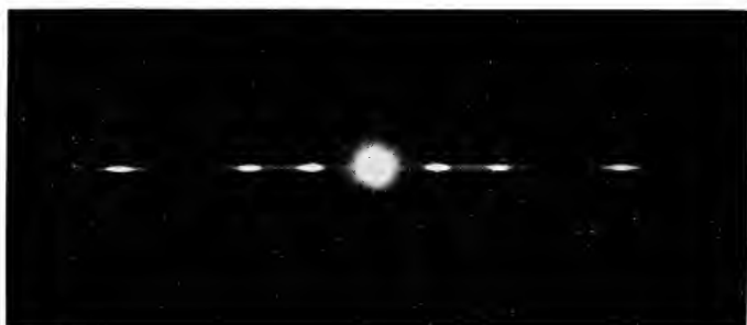
Fig. 5.—Spectrum formed by the grid of the 1553 microwave triode.
