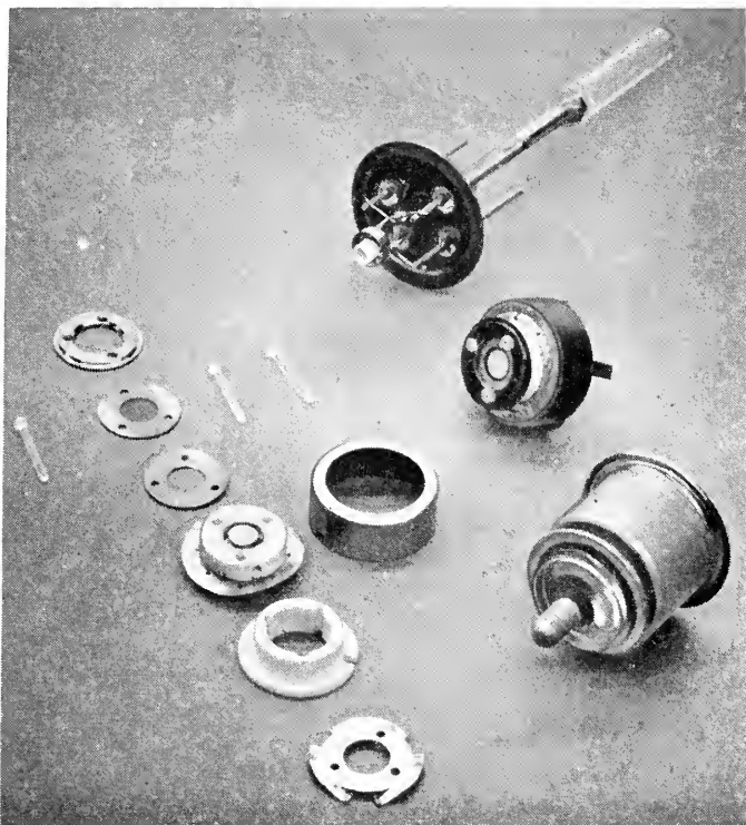
Fig. 4.—Physical appearance of the elements comprising the 1553 triode.
