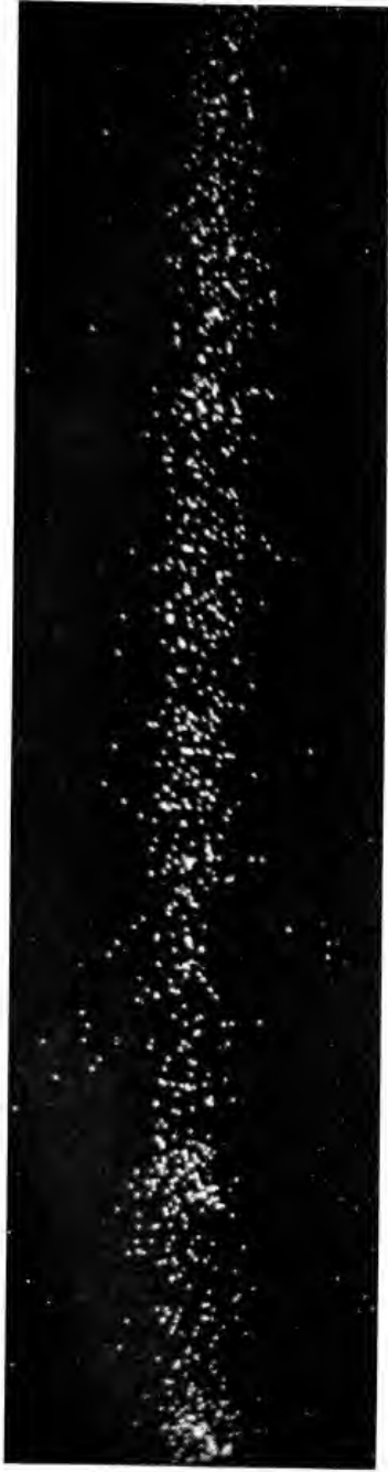
Fig. 1—Track of a cosmic-ray particle (probably an electron) in the expansion-chamber, time having been allowed for the ions to drift apart before the expansion. (Corson and Brode, University of California)
