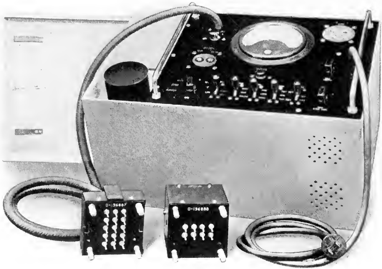
Fig. 13—Outlying-station test set.
