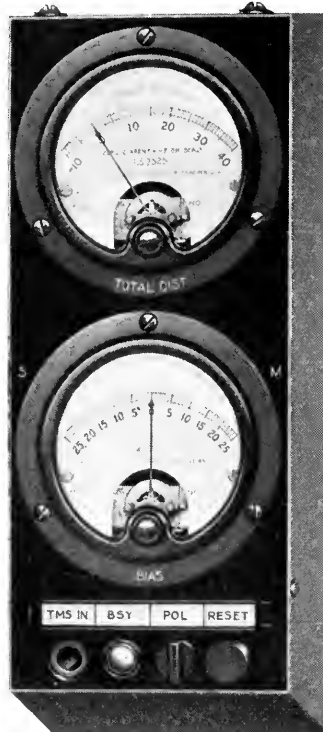
Fig. 3—Meters and control apparatus at telegraph board.
