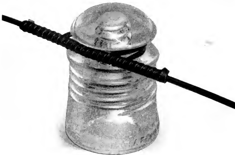
Fig. 4—Flat tie wire shown as installed.
