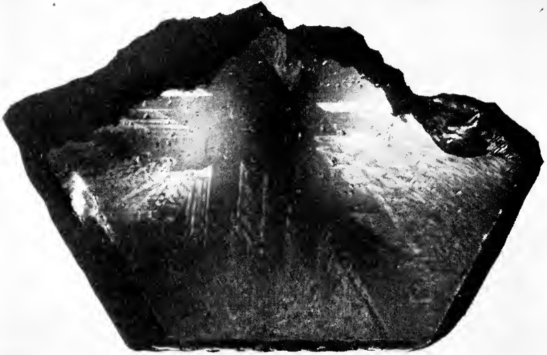
Fig. 3—Right and left-hand twinning in quartz as seen by polarized light.
