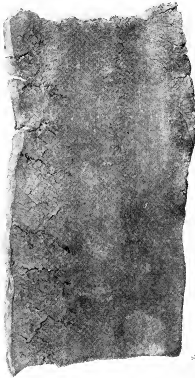
Fig. 2—View of piece of old cable sheath made of commercially pure lead, which failed in service from intercrystalline fracture.
