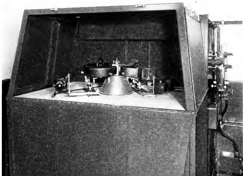
Fig. 5—X-ray diffraction apparatus showing cameras mounted for identification of structure and precision measurement of lattice constant.
