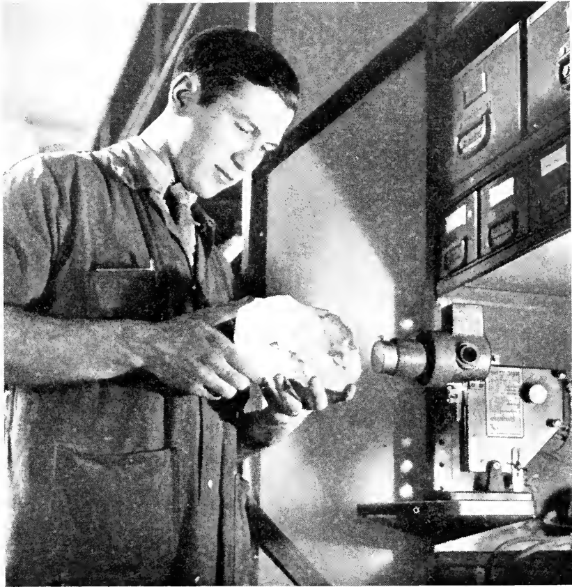
Fig. 2—Inspection of quartz crystals. An arc light beam aids in the detection of internal flaws.
