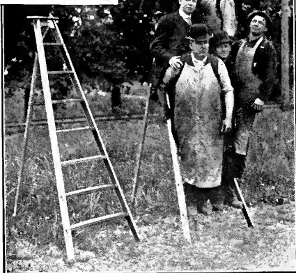
Weight of ladder 32 pounds Weight of load 1397 pounds
