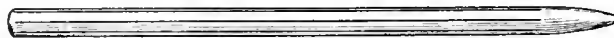
Fig. 2. Punch for making the bore holes. This is driven in with a heavy hammer.
