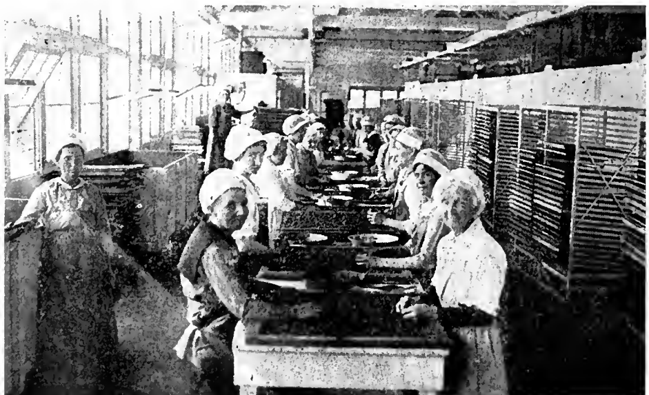
Spreading loganberries on trays preparatory to being dehydrated. To the right can be seen the partially loaded steel cars which are used in routing the food materials through the plant.
