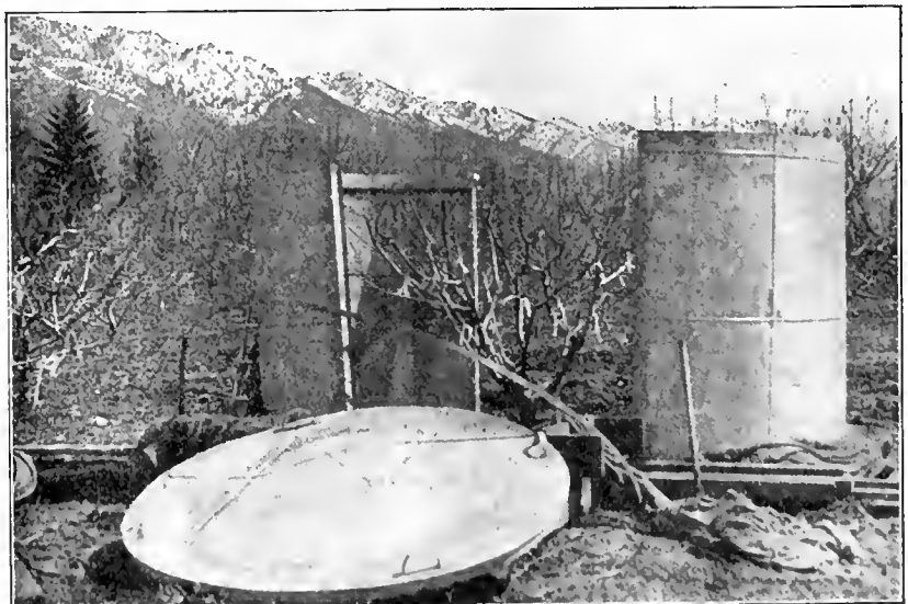
Apparatus used in freezing entire tree in experiments made at the Utah Agricultural Experiment Station, to determine the temperatures at which fruit buds are damaged by frost.
