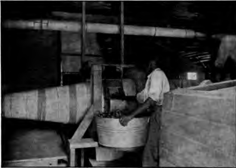
FIG. 15.—Loading end of sterilizer to destroy enzymes. (Bureau of Plant Industry, U. S. Dept. of Agriculture.)
