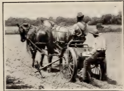
A MACHINE POTATO-PLANTER OPENS THE FURROWS, PLANTS THE SEED, COVERS IT AND MARKS THE NEXT ROW
