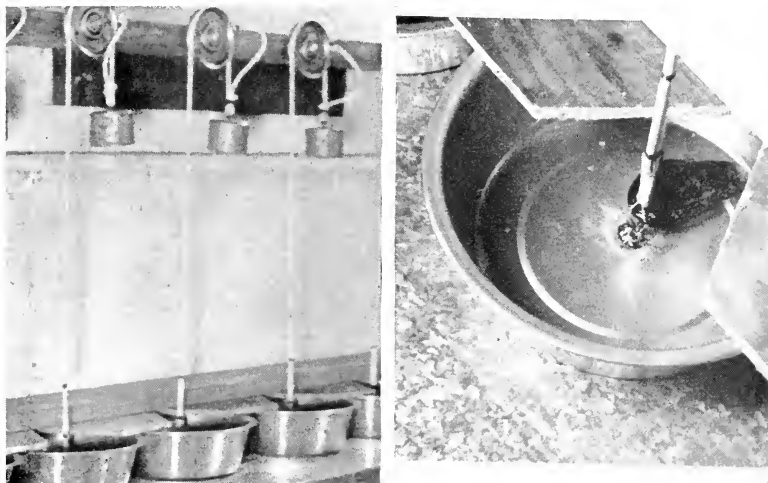
FIGURE 1. Constant stress apparatus. Each 800-gram weight was suspended by a cord passing over a ball-bearing pulley to a double hook inserted into notches filed in the beak of the mussel shell. Another hook, also made from two bent pins, was soldered to the bottom of the pan and passed through the same notches. Gapes were measured by means of a calibrated metal triangle which could be slipped in between the valves near the hooks.
