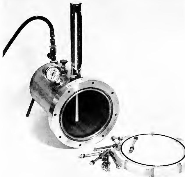
FIGURE 1. Compressor unit (4.4 l capacity) for experiments on upper lethal temperature at high tensions of oxygen. Chamber is constructed of stainless steel, with perspex end plate. Thermometer, pressure gauge, bleeder valve and high pressure oxygen hose are shown.
