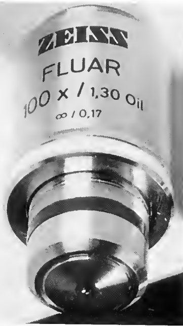
Figure 1. An objective lens with typical markings. Although this is a Zeiss lens, most manufacturers use similar markings.
