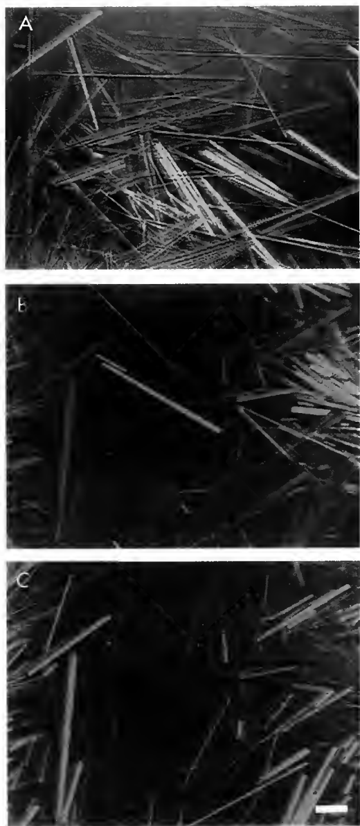
Figure 1. Crystals of purified native GFP. (A) Dichroism (anisotropic absorbance) in visible light with crystals appearing green to light brown with the long crystal axis oriented "parallel," and pale blue to white with the long crystal axis oriented "perpendicular," to the polarizer. (In fact, a polarizer and analyzer were used, off-crossed by about five degrees, to accentuate the weak visible light dichroism.) (B, C) Polarization-dependent anisotropy of fluorescence excitation seen in the absence of an analyzer. The polarizer E-vector in Panel B is oriented parallel to the prominent crystal in the middle of the panel. In Panel C, it is oriented perpendicular to the length of the same crystal. Bar = 30 \mu\text{m} .
