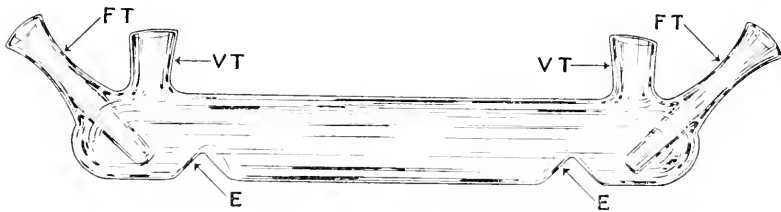
FIG. 1. Type of sperm tube used. FT , feed tube; VT , ventilating tube; E , elevation in the floor of the sperm tube.
