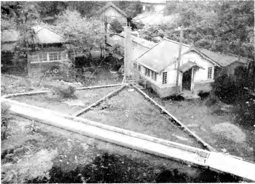
FIG. 3. General view of pilot-plant for Chlorella production designed and built by Arthur D. Little, Inc., Cambridge, Mass. Note plastic cover to photosynthesizing trough and large vertical tower for treating culture medium with \text{CO}_2 gas.
