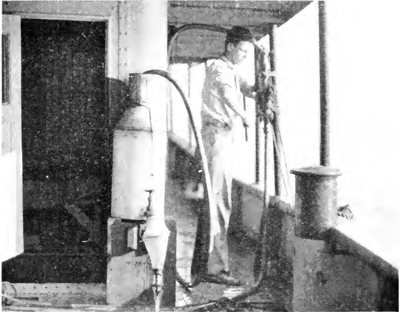
Pump arrangement for net plankton
