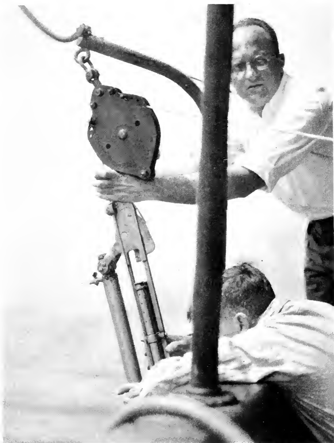
Greene-Bigelow water bottle with Richter reversing thermometer
