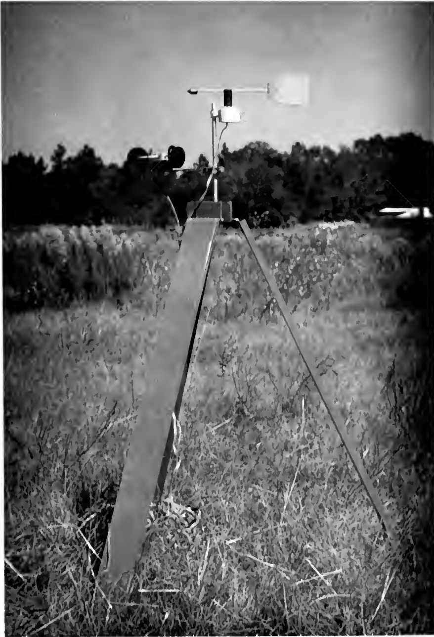
Figure 15. Wind vane and anemometer mounted on tripod for observations.
