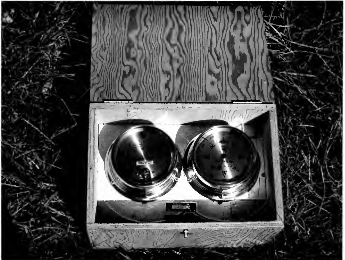
Figure 14. Wind speed and direction dials used in migration studies.
