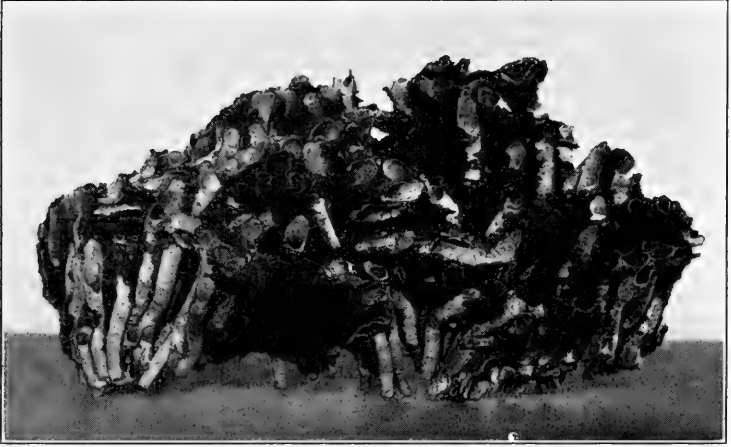
I.—TIMBER BORED BY THE SHIP-WORM ( Teredo norvegica ).
