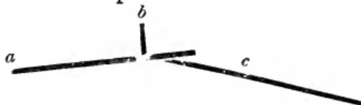
horizontal line *a* the shaft of the cart, the perpendicular one *b* the shaft-horse's back-band, and the declining one *c* the front horse's trace ; the pressure on the back
