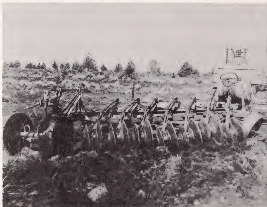
Figure 3.--The brushland plow in action on the Flukey Well 18 acre pilot planting in the spring of 1957. Before plowing, the heavy brush was removed with a brush blade mounted on this same tractor.
