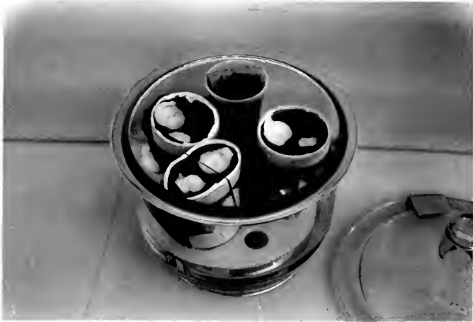
Figure 6. Glass container and paper cartons used for holding black fly adults alive in the laboratory.
