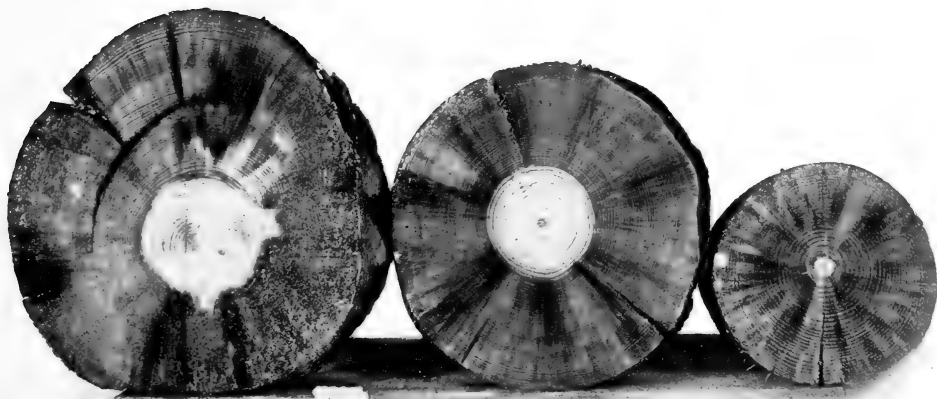
FIG. 2.—SECTIONS FROM TREE DEAD EIGHTEEN MONTHS. "BLUE" SECTIONS FROM DEAD TREES.
