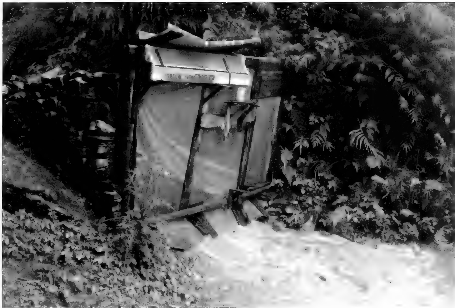
Fig. 2. Emergence trap at Naggar Nala during the summer monsoon (photo by A. Stauder).
