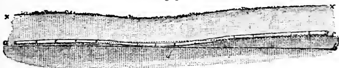
Defective Grade, resulting from Uniform Depth.
